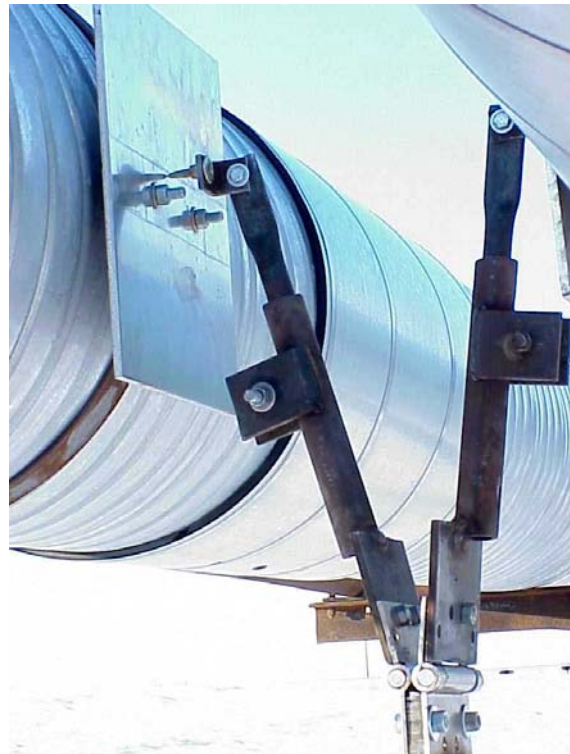
Figure 1 Typical Installation of Scratch Gages for Alpine Pipelines
