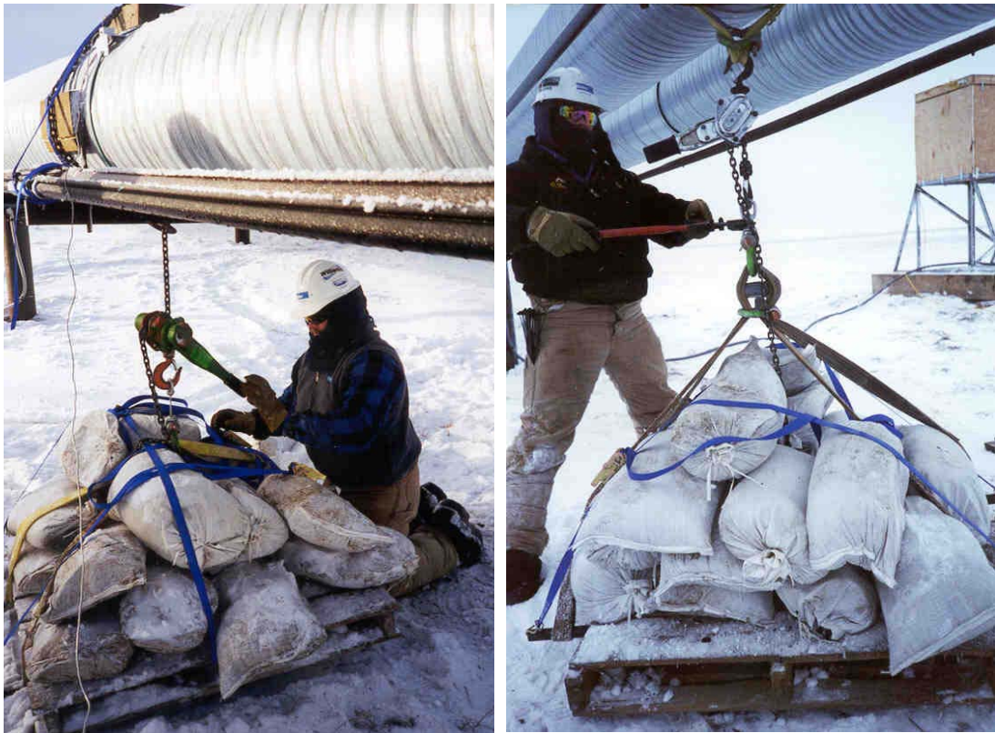
Figure 3 Jacking Reaction Weight and Releasing to Initiate Free-Vibration
